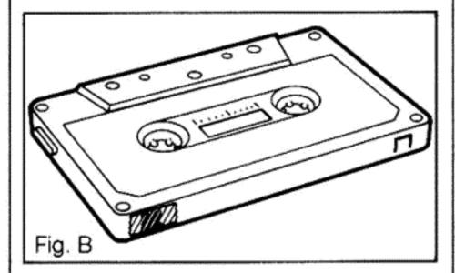
To record on a cassette that has had the tab(s) removed, cover the slot with a quality masking tape, then record in the usual manner. To avoid fouling the cassette and deck parts with adhesive, remove the masking tape immediately after recording.
