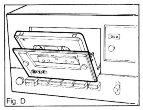
NOTE: When a cassette has been stored for a period of time, it is a good practice to run it through FAST FORWARD and then REWIND. This will eliminate any static charge or sticking of the tape. Your B·I·C will perform this operation considerably faster than most other cassette decks.
